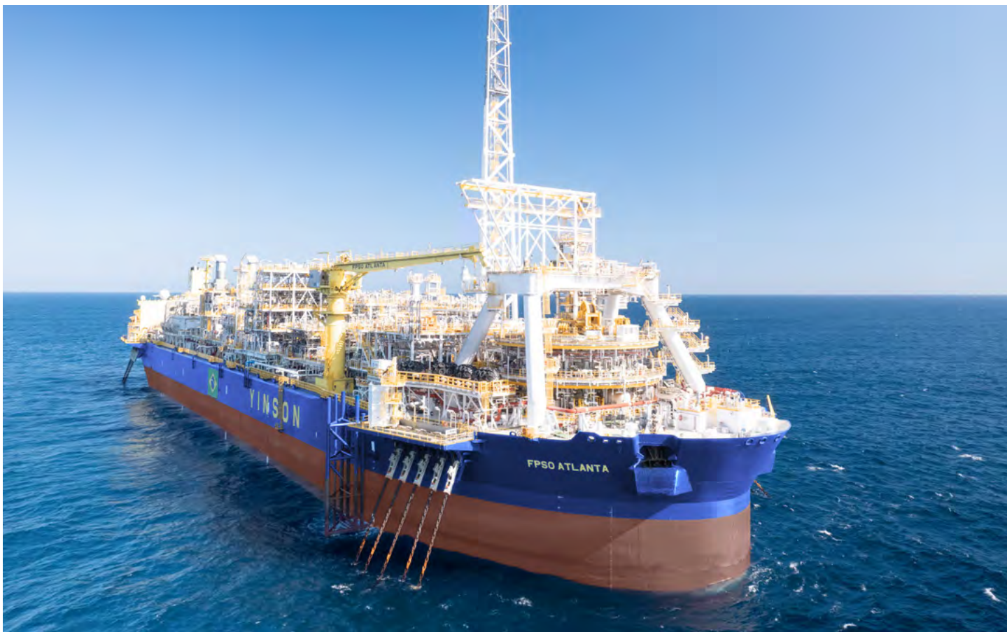
The FPSO Atlanta, stationed 185 km offshore in the Santos Basin, serves as the heart of Atlanta Field's production system, capable of processing up to 50,000 barrels per day of heavy crude.
